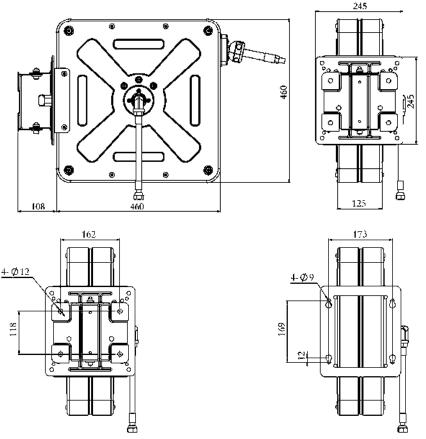
Mounting Holes With Swivel Base Plate
